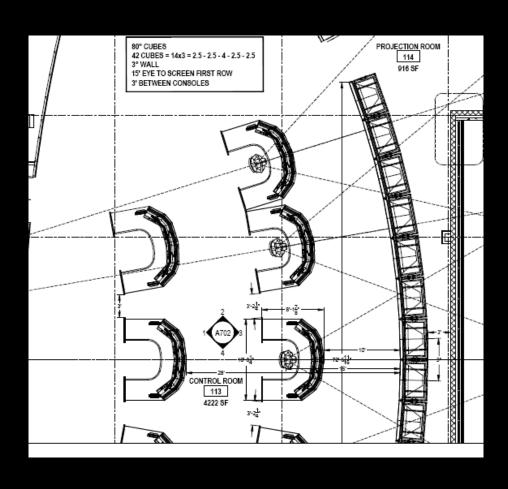
All angles checked against ISO 11064 specification & specifically for Barco Displays.
