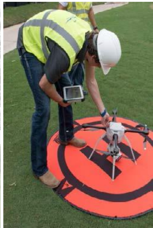
Figure 10.10: Use of drones to perform inspections.
