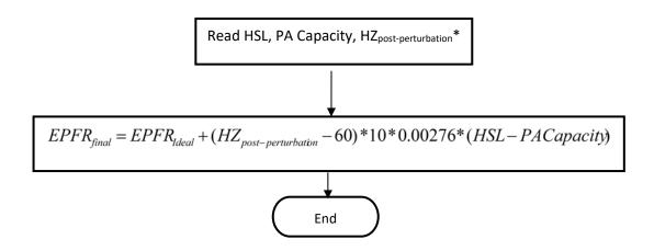
0.00276 is the MW/0.1 Hz change per MW of Capacity and represents the MW change in generator output due to the change in mass flow through the combustion turbine due to the speed change of the turbine during the post-perturbation measurement period. (This factor is based on empirical data from a major 2003 event as measured on multiple combustion turbines in ERCOT.)
