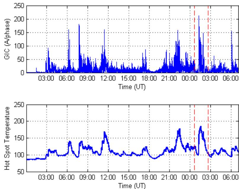
**Figure 10: Magnitude of GIC(t) and Metallic Hot Spot Temperature  $\theta(t)$  Assuming Full Load Oil Temperature of 85.3°C (40°C ambient). Dashed lines approximately show the close-up area for subsequent Figures.**
