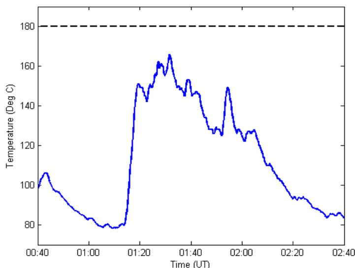
**Figure 11: Close-up of Metallic Hot Spot Temperature Assuming a 75% Load**
