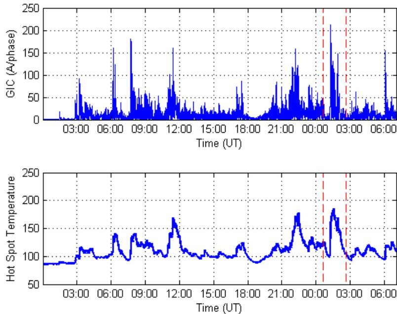
**Figure 9: Magnitude of GIC(t) and Metallic Hot Spot Temperature  $\theta(t)$  Assuming Full Load Oil Temperature of 85.3°C (40°C ambient). Dashed lines approximately show the close-up area for subsequent Figures.**
