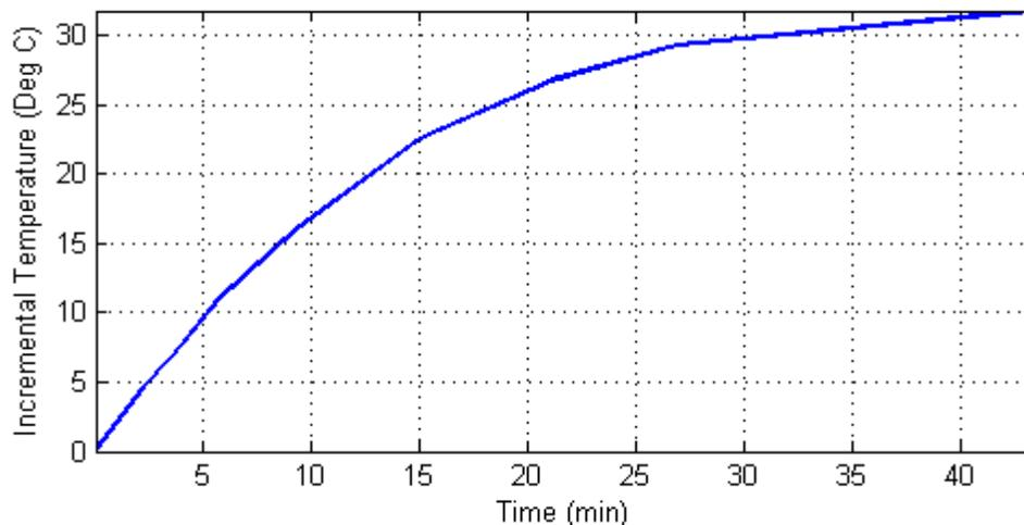
**Figure 7: Thermal Step Response to a 16.67 Amperes per Phase dc Step**
