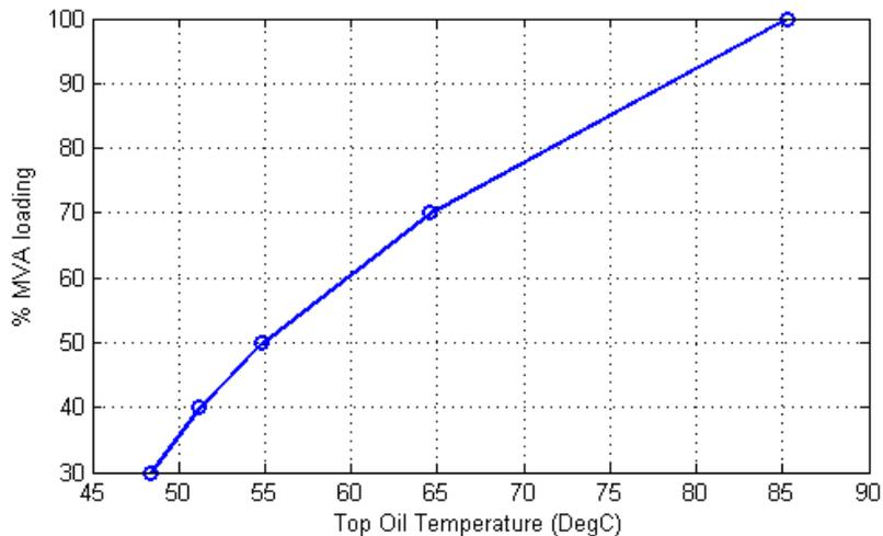
**Figure 13: Simplified Loading Curve Assuming 40°C Ambient Temperature.**
