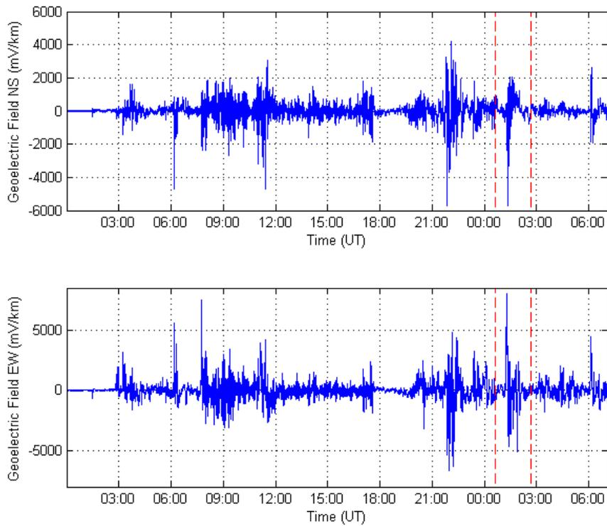
**Figure 4: Calculated Geoelectric Field  $E_N(t)$  and  $E_E(t)$  Assuming  $\alpha=1$  and  $\beta=1$  (Reference Earth Model).** Zoom area for subsequent graphs is highlighted. Dashed lines approximately show the close-up area for subsequent Figures.
