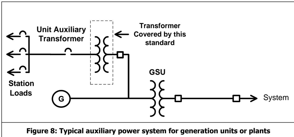
**Figure 8: Typical auxiliary power system for generation units or plants**
