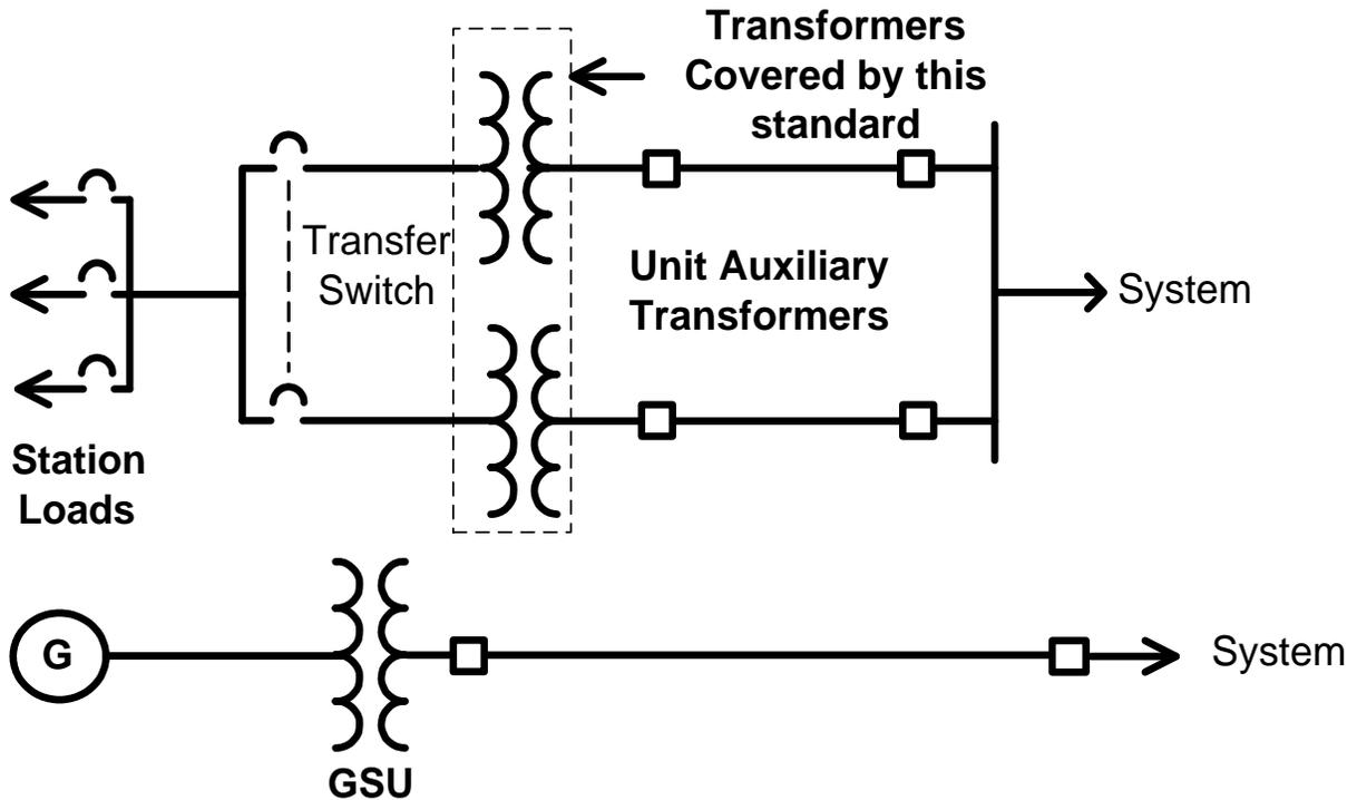
**Figure 7: Auxiliary Power System (independent from generator)**
