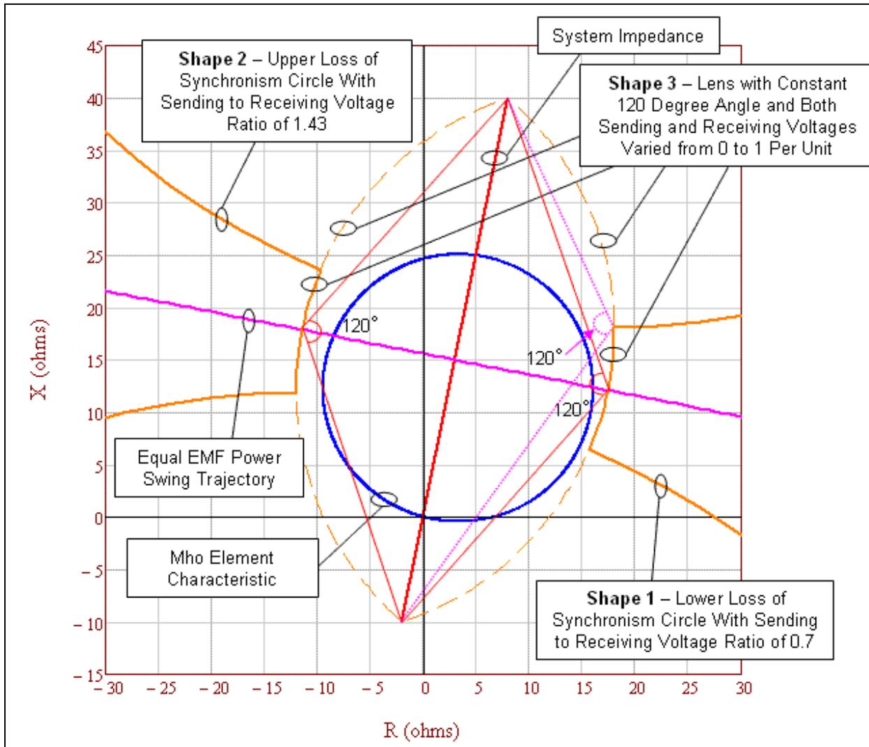
**Figure 1:** An enlarged graphic illustrating the unstable power swing region formed by the union of three shapes in the impedance (R-X) plane: Shape 1) Lower loss-of-synchronism circle, Shape 2) Upper loss-of-synchronism circle, and Shape 3) Lens. The mho element characteristic is completely contained within the unstable power swing region (i.e., it does not intersect any portion of the unstable power swing region), therefore it meets PRC-026-1-2 – Attachment B, Criterion A, No. 1.
