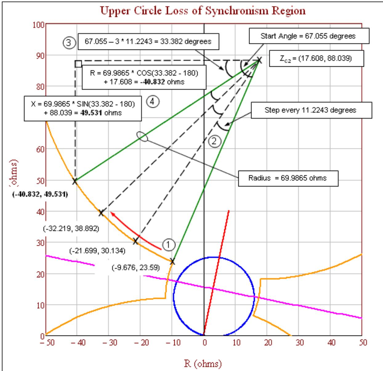
**Figure 15h:** Upper circle loss-of-synchronism region showing the final steps to calculate the coordinates of the points on the circle. 1) Start at the intersection with the lens shape and proceed in a clockwise direction. 2) Advance the step angle for each point. 3) Calculate the new angle after step advancement. 4) Calculate the R-X coordinates.
