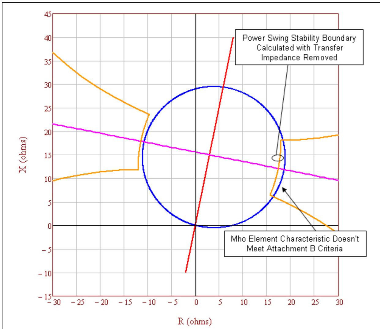
**Figure 10:** This is an example of an unstable power swing region (i.e., the orange characteristic) with the parallel transfer impedance removed. This relay mho element characteristic (i.e., the blue circle) does not meet PRC-026-1 Attachment B, Criterion A because it is not completely contained within the unstable power swing region.
