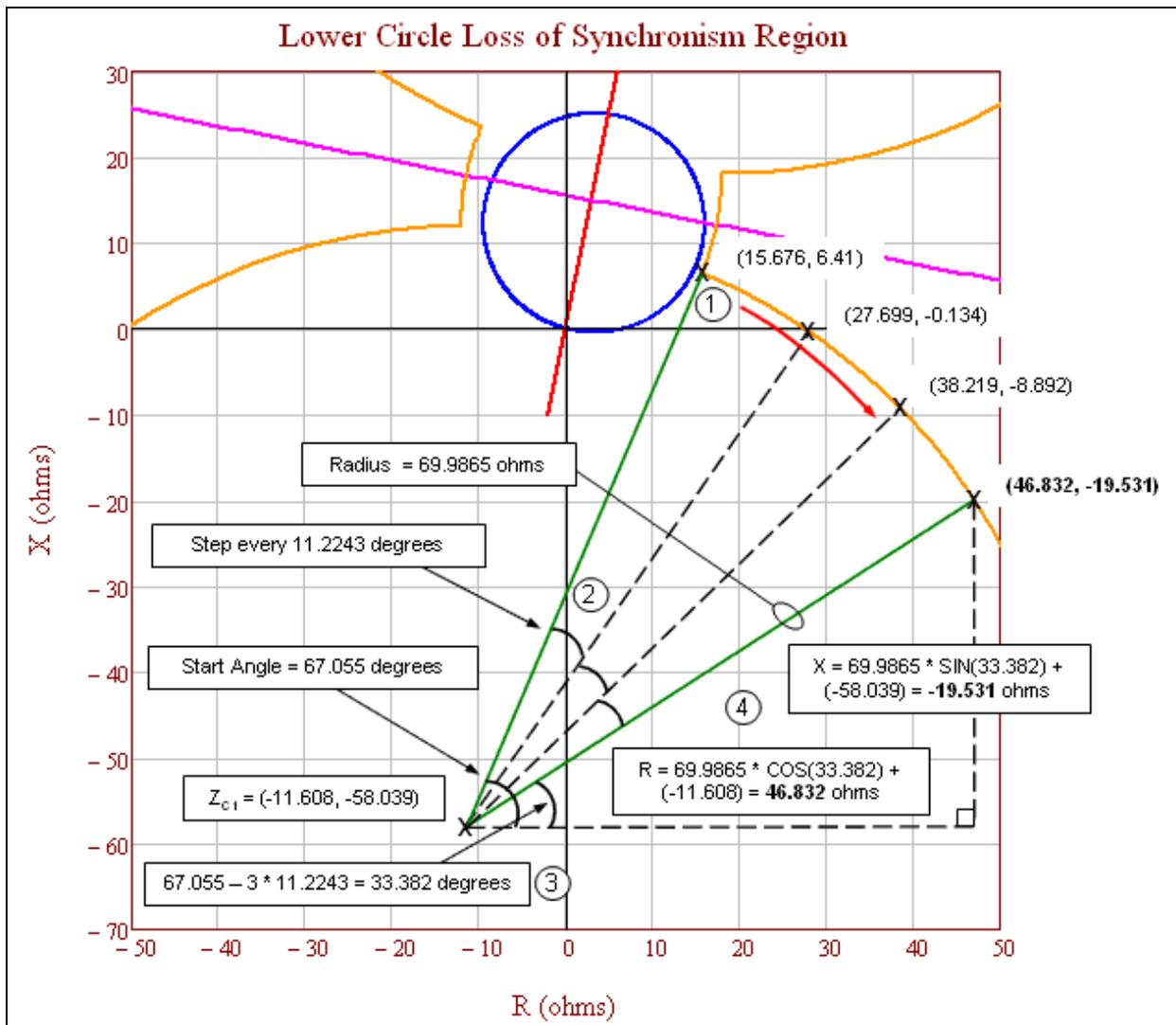
**Figure 15d:** Lower circle loss-of-synchronism region showing the final steps to calculate the coordinates of the points on the circle. 1) Start at the intersection with the lens shape and proceed in a clockwise direction. 2) Advance the step angle for each point. 3) Calculate the new angle after step advancement. 4) Calculate the R–X coordinates.
