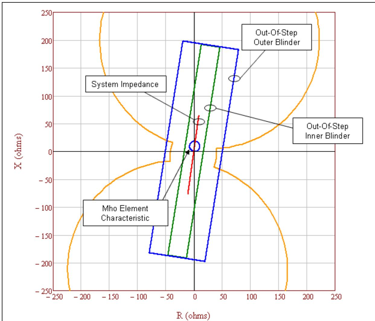
**Figure 15:** Out-of-step trip (OST) inner blinder (i.e., the parallel green lines) meets the PRC-026-1.2 – Attachment B, Criterion A because the inner OST blinder initiates tripping either On-The-Way-In or On-The-Way-Out. Since the inner blinder is completely contained within the unstable power swing region (i.e., the orange characteristic), it meets the PRC-026-1.2 – Attachment B, Criterion A.
