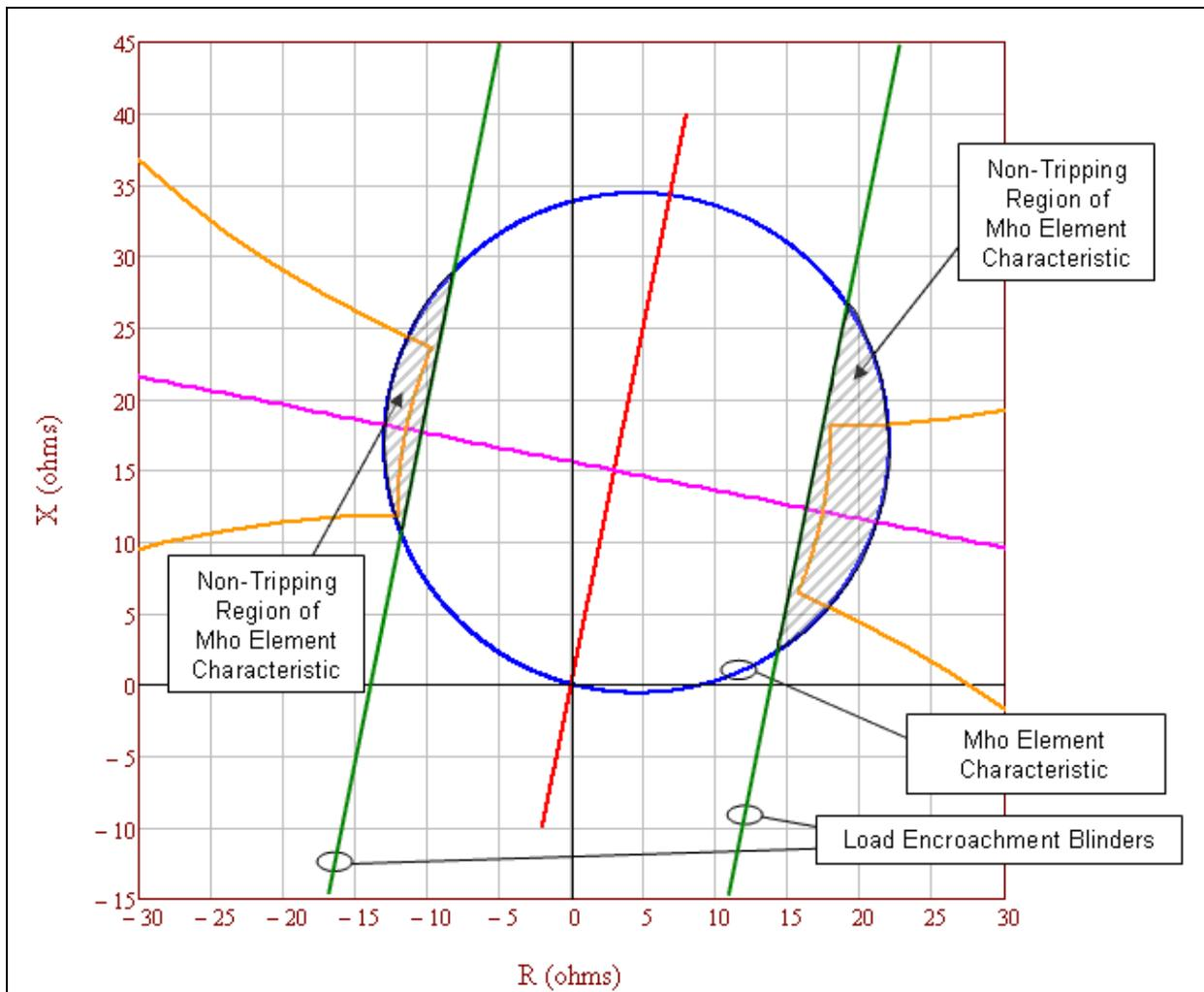
**Figure 12:** The tripping portion of the mho element characteristic (i.e., the blue circle) not blocked by load encroachment (i.e., the parallel green lines) is completely contained within the unstable power swing region (i.e., the orange characteristic). Therefore, the mho element characteristic meets the PRC-026-1-2 Attachment B, Criterion A.
