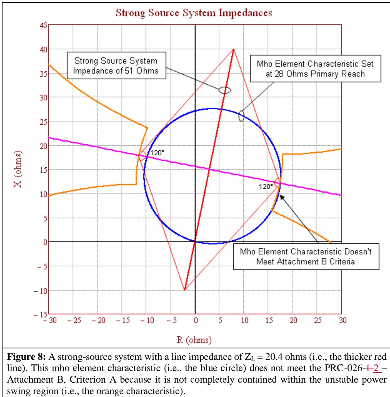
**Figure 8:** A strong-source system with a line impedance of  $Z_L = 20.4$  ohms (i.e., the thicker red line). This mho element characteristic (i.e., the blue circle) does not meet the PRC-026-1-2 – Attachment B, Criterion A because it is not completely contained within the unstable power swing region (i.e., the orange characteristic).
