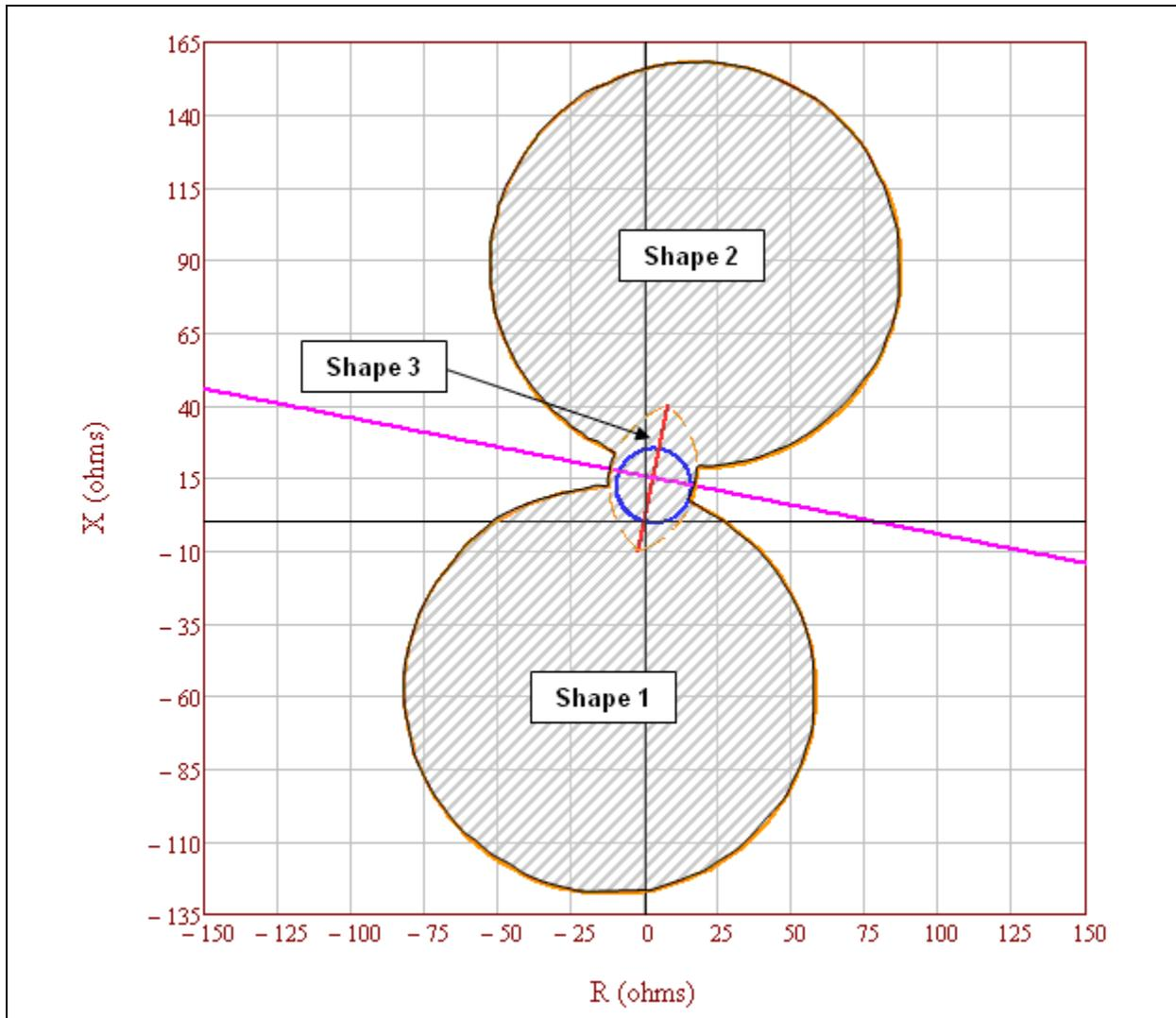
**Figure 2:** Full graphic of the unstable power swing region formed by the union of the three shapes in the impedance (R-X) plane: Shape 1) Lower loss-of-synchronism circle, Shape 2) Upper loss-of-synchronism circle, and Shape 3) Lens. The mho element characteristic is completely contained within the unstable power swing region, therefore it meets PRC-26-1 – Attachment B, Criterion A, No.1.
