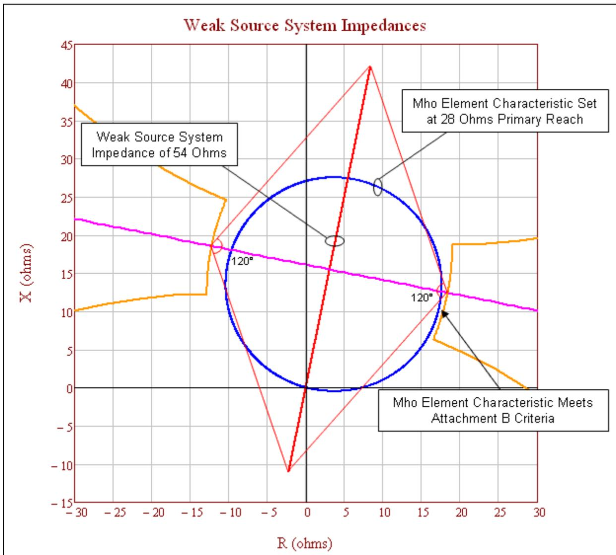
**Figure 9:** A weak-source system with a line impedance of  $Z_L = 20.4$  ohms (i.e., the thicker red line). This mho element characteristic (i.e., the blue circle) meets the PRC-026-1 Attachment B, Criterion A because it is completely contained within the unstable power swing region (i.e., the orange characteristic).
