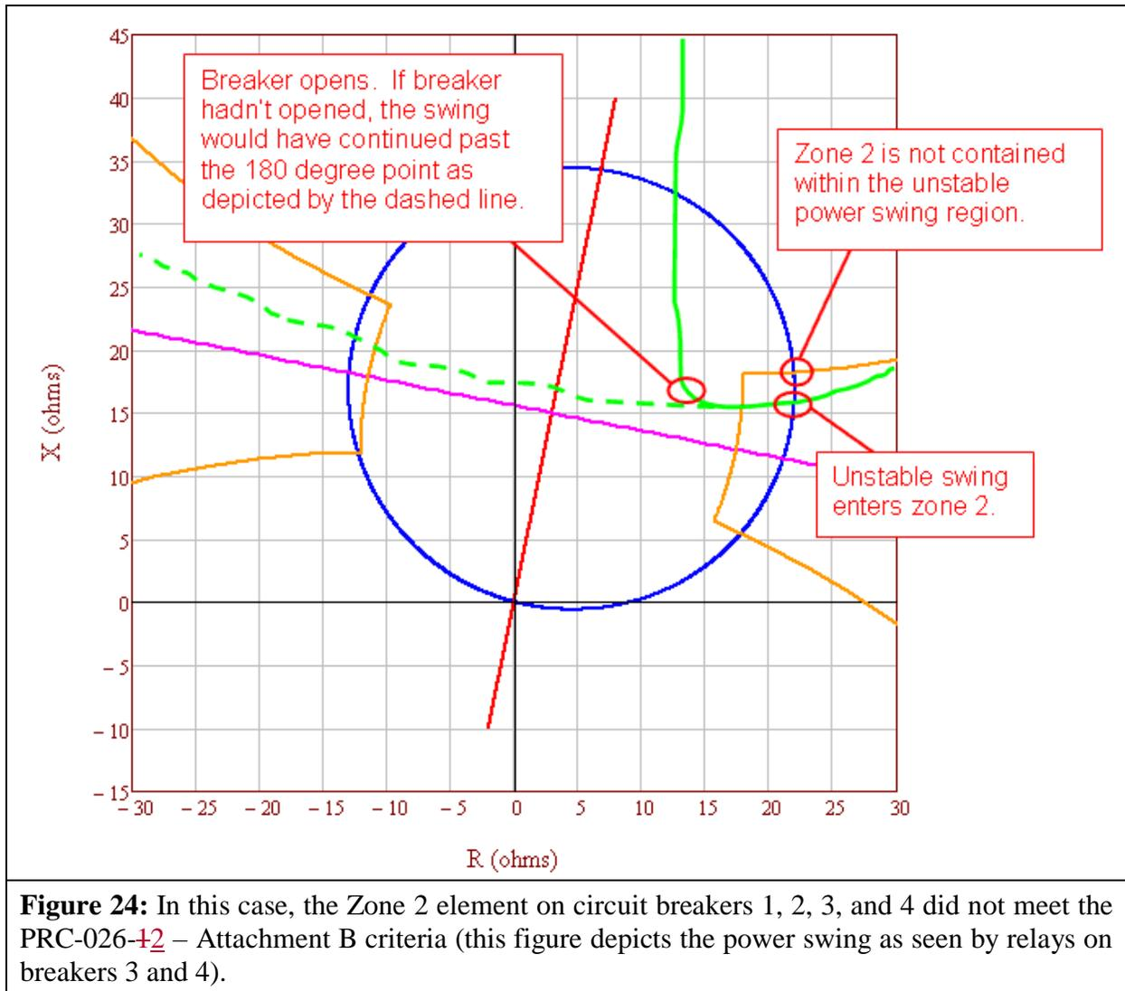
In Figure 24, a large disturbance occurs within the small utility and its system goes out-of-step with the large interconnect. The small utility is importing power at the time of the disturbance. The actual power swing, as shown by the solid green line, enters the Zone 2 relay characteristic on the terminals of Lines 1, 2, 3, and 4 causing both lines to trip as shown in Figure 25.
