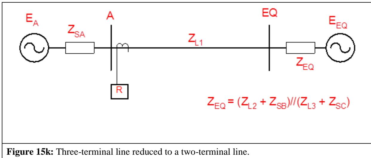
**Figure 15k:** Three-terminal line reduced to a two-terminal line.
