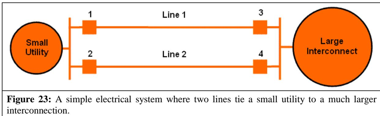
**Figure 23:** A simple electrical system where two lines tie a small utility to a much larger interconnection.
