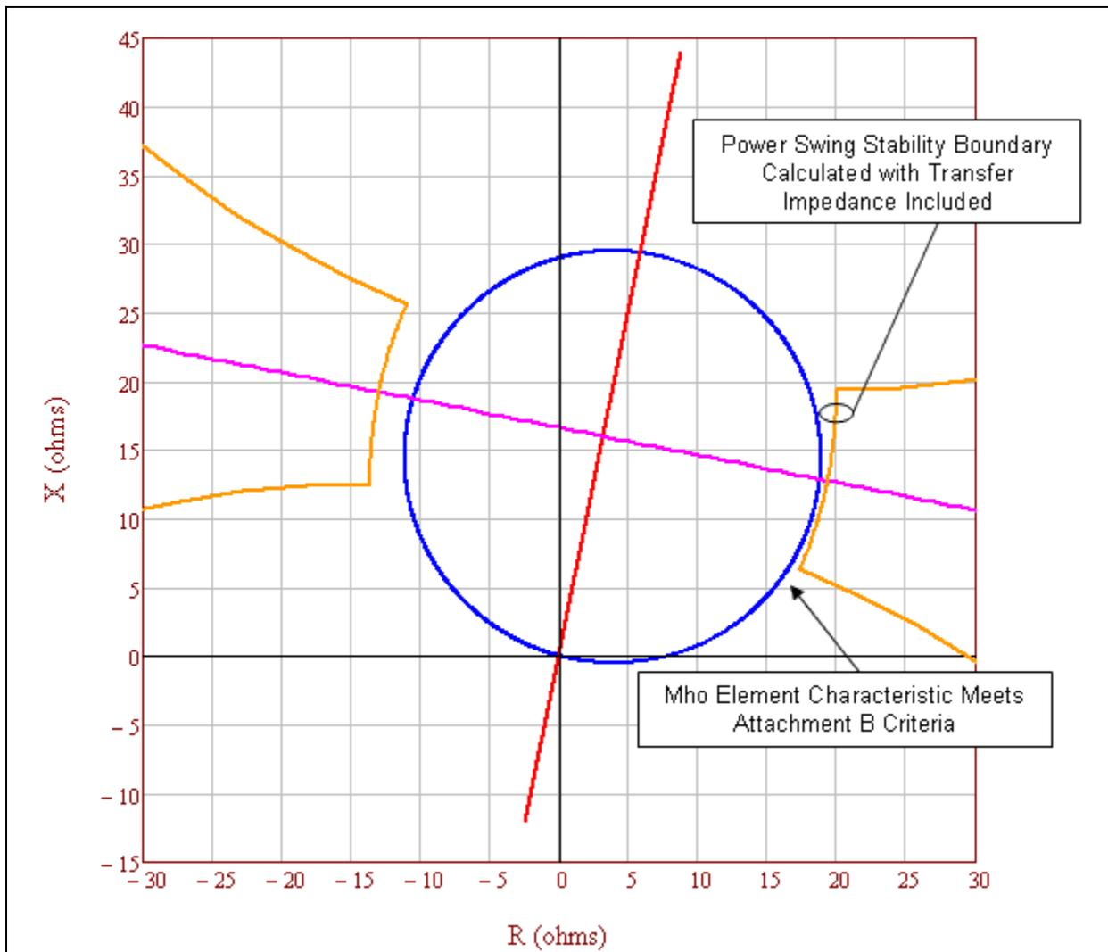
**Figure 11:** This is an example of an unstable power swing region (i.e., the orange characteristic) with the parallel transfer impedance included causing the mho element characteristic (i.e., the blue circle) to appear to meet the PRC-026-1-2 Attachment B, Criterion A because it is completely contained within the unstable power swing region. Including the parallel transfer impedance in the calculation is not allowed by the PRC-026-1-2 Attachment B, Criterion A.
