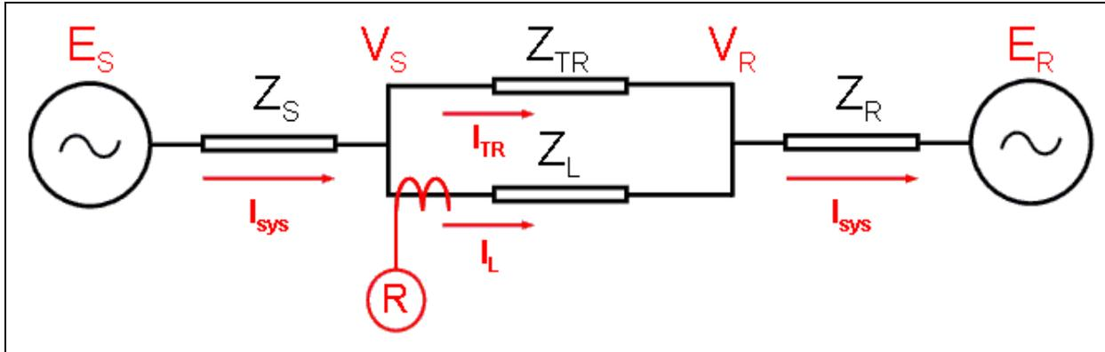
**Figure 13:** The infeed diagram shows the impedance in front of the relay R with the parallel transfer impedance included. As the parallel transfer impedance approaches infinity, the impedances seen by the relay R in the forward direction becomes  $Z_L + Z_R$ .
