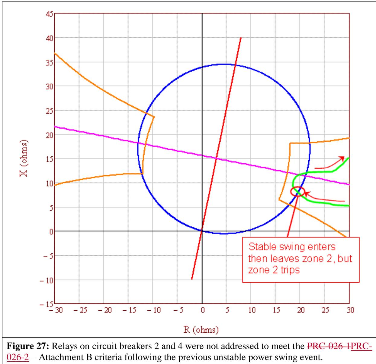
If the relays on circuit breakers 2 and 4 were not addressed under the Requirements for the previous unstable power swing condition, the relays would trip in response to the stable power swing, which would result in unnecessary system separation, load shedding, and possibly cascading or blackout.
