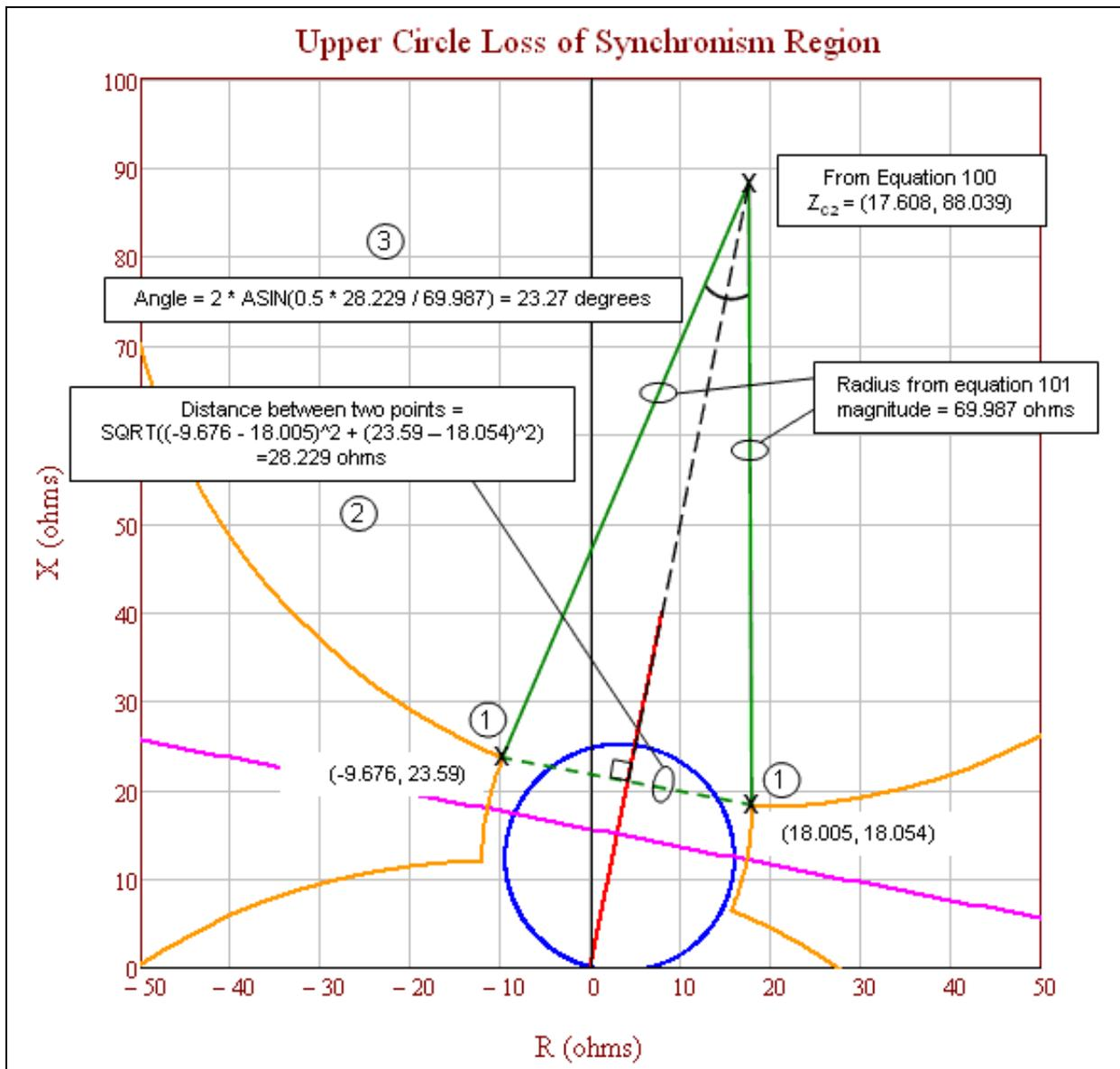
**Figure 15f:** Upper circle loss-of-synchronism region showing the first three steps to calculate the coordinates of the points on the circle. 1) Identify the upper circle points that intersect the lens shape where the sending-end to receiving-end voltage ratio is 1.43 (see lens shape calculations in Tables 2-7). 2) Calculate the distance between the two upper circle points identified in Step 1. 3) Calculate the angle of arc that connects the two upper circle points identified in Step 1.
