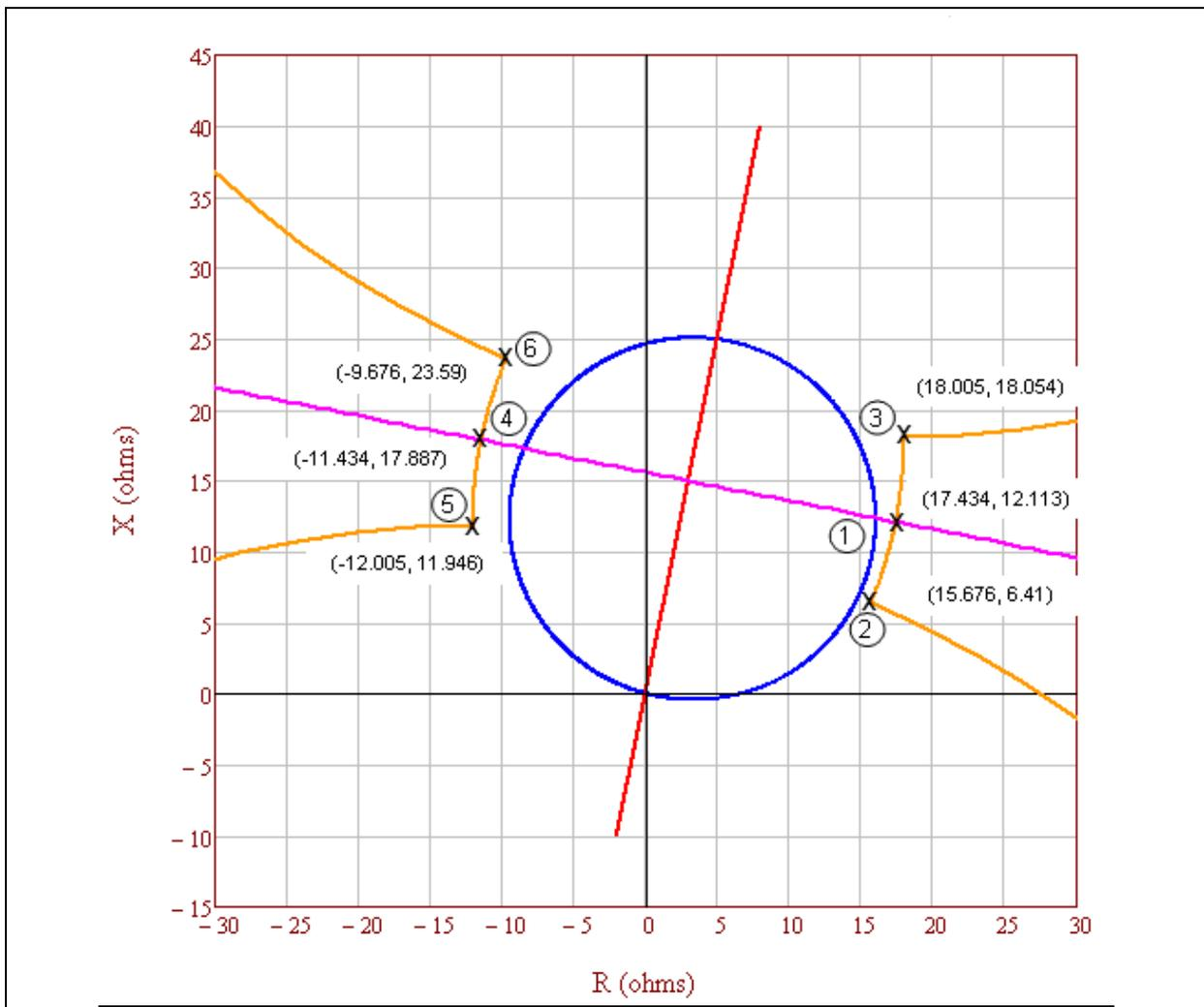
**Figure 4:** The defining unstable power swing region points where the lens shape intersects the lower and upper loss-of-synchronism circle shapes and where the lens intersects the equal EMF (electromotive force) power swing.
