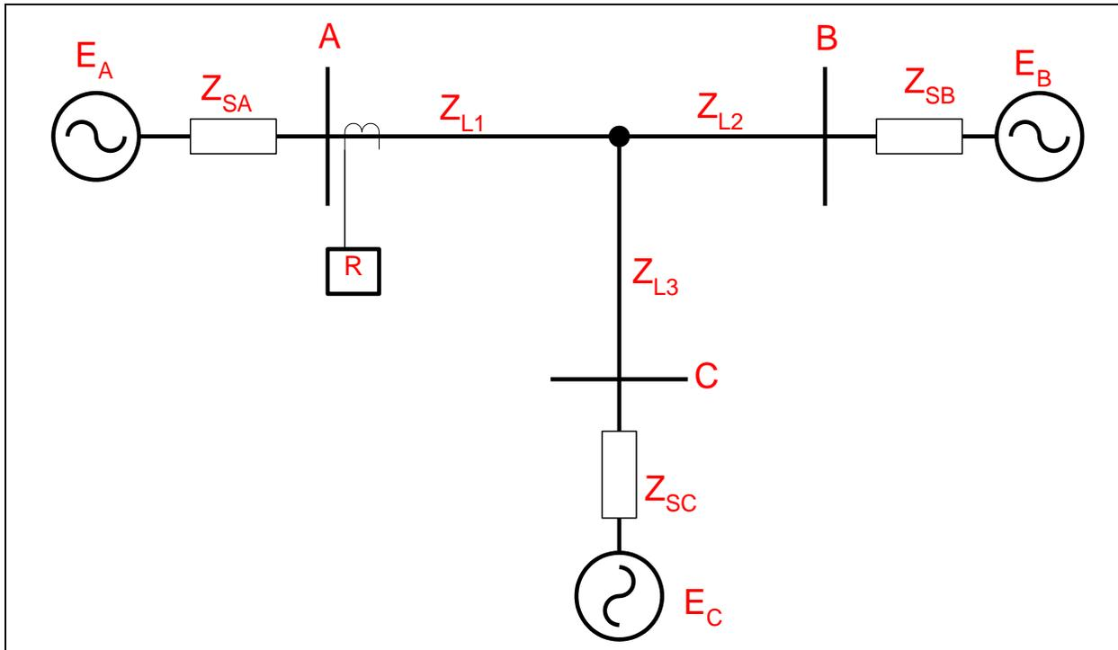
**Figure 15j:** Three-terminal line. To evaluate the load-responsive protective relays on the three-terminal line at Terminal A, the circuit in Figure 15j is first reduced to the equivalent circuit shown in Figure 15k. The evaluation process for the load-responsive protective relays on the line at Terminal A will now be the same as that of the two-terminal line.
