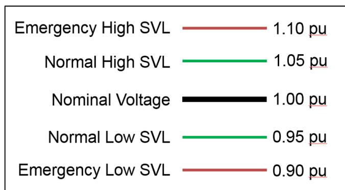
**Figure 6. Example of a System Voltage Limit Set**
