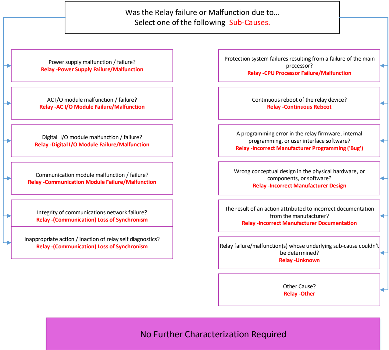
Figure H.9: Relay Failure/Malfunction Sub Cause of Misoperation
