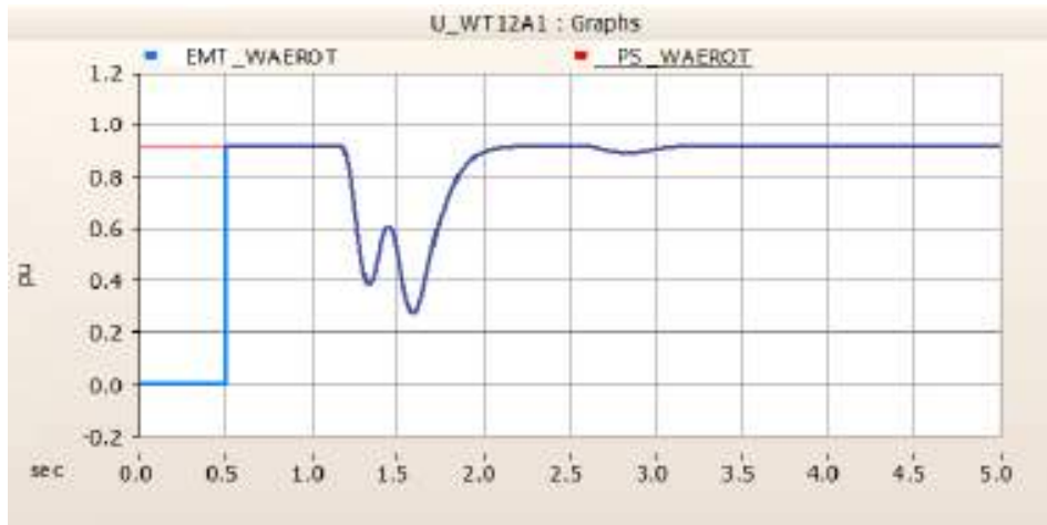
Figure A.4: Comparison of WT12A1 Responses Between EMT and Positive-Sequence Simulation
