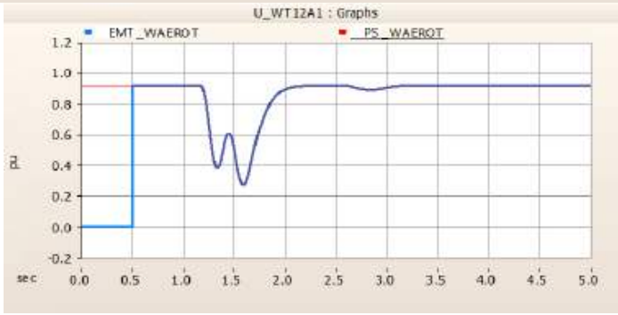
Figure A.4:- Comparison of WT12A1 responses between EMT and Positive Sequence simulation
