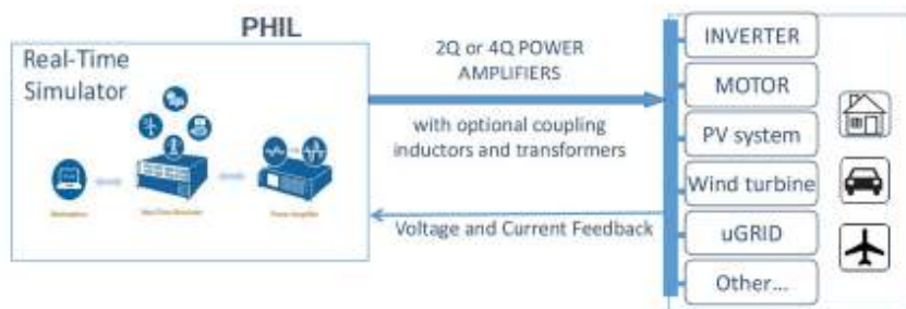
Figure 7.2: PHIL setup to interface electric components
