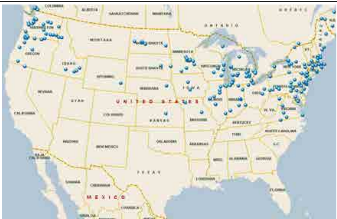
Figure 2-6- Location of At-Risk Transformers for 4800 nT/min at 55° (GIC > 90 Amps/phase).
