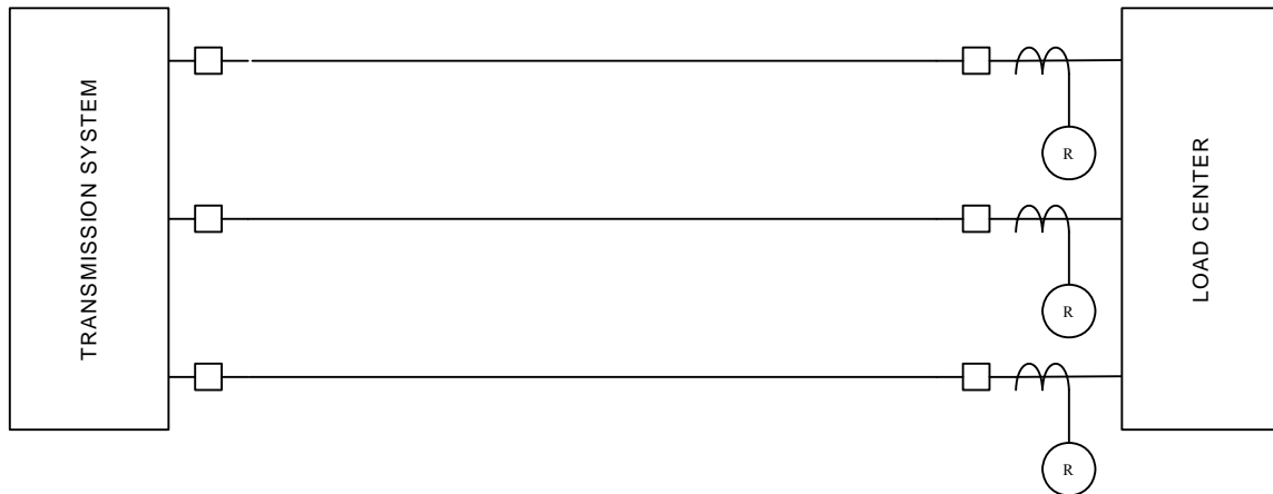
Figure 9 –Load Center Remote to Transmission System
